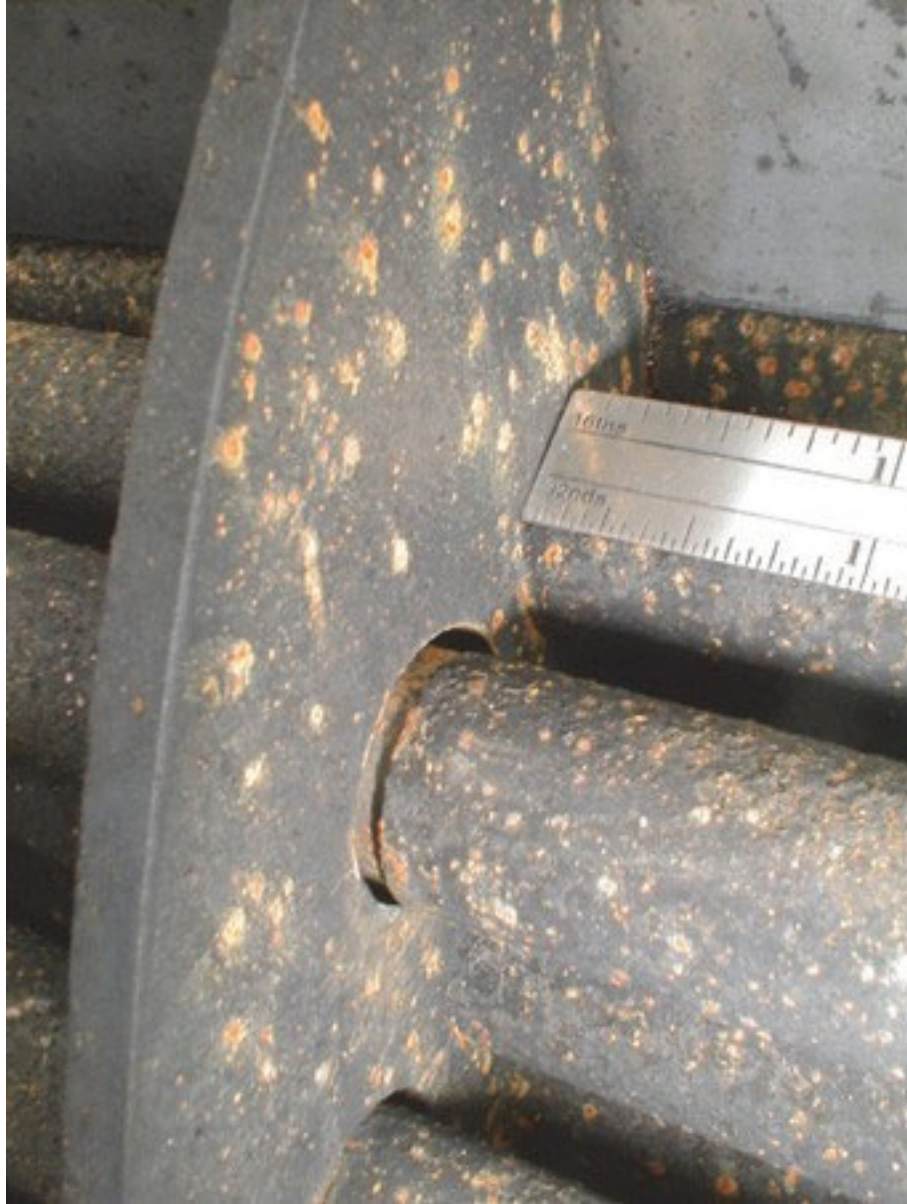
Figure A.4 - Tubes Thinned at Baffles
